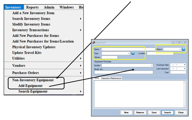
Enter as much information about the piece of equipment as you would like. The requirements to save an entry are Name and Status, Type and Abbreviation, the other fields are optional. Complete the entry, with as much detail and hit save. That will create the Equipment.
